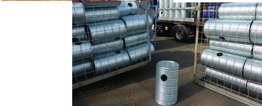
**Folded spiral-seam pipe of zinc-coated sheet metal**
